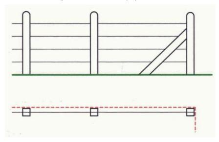
The upper part of the above drawing shows a strainer fence, so called because of the diagonal strainer placed against the terminal post at either end of the fence to counteract the tension in the wires that might otherwise pull the terminal posts over. The lower part of the image is the same fence shown in plan view. It is tempting to deduce that two faces of the terminal post each stand against a boundary, as shown by the red dashed lines.
